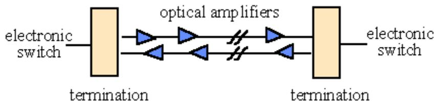
The link provided a 622 Mbps channel for use by the testbed in both directions between Madison and Champaign, and in addition was shared with other AT&T operational services using other capacity available on the optical link. This was the first deployment of optical fiber amplifiers as repeaters on a service basis by a carrier. The testbed-based link deployment allowed data to be collected by AT&T on link dispersion, signal-to-noise ratio, and bit error rates.
