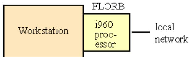
Their design consisted of a shared fast SRAM, a single Intel 960 RISC processor, a FIFO at each of the four host and network input and output ports, and a DMA controller. A novel aspect of their design concerns the way in which the processor controls the data bus, allowing data to be
