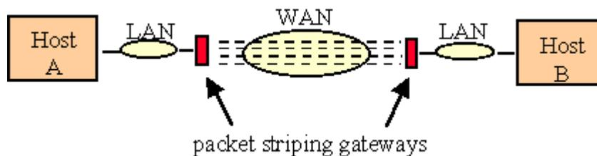
Consideration of equipment design complexity and cost associated with the choice of byte, cell, and packet striping units led to the selection of a packet striping unit, where packets in the initial implementation consisted of HIPPI frames. A distinct ATM VC is used for each 155 Mbps stripe, with the HIPPI frames which are received on the set of VCs sequentially combined into
