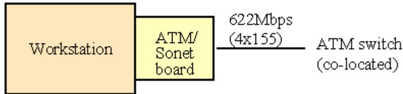
A key question for the board-level approaches was how much functionality should be handled by specialized hardware and software on the board itself, and how much should be done by software using the workstation's main processor (while leaving enough processor bandwidth to also run applications).
