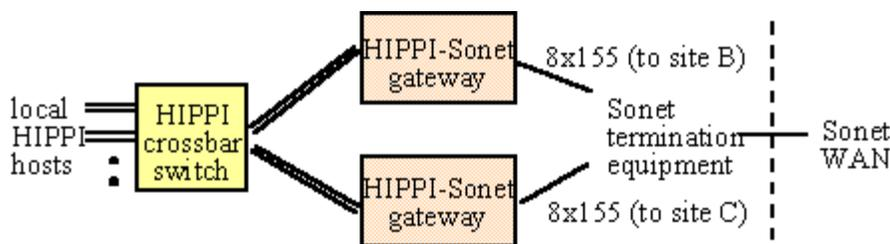
Buffering in the gateways and hosts allowed Casa to be operated as a store-and-forward packet switched network over its wide area end-to-end paths, in spite of the absence of buffering in the HIPPI switches. Routing was accomplished by defining a logical network-wide address for each host in the network and configuring a logical-physical address mapping table in each switch.
