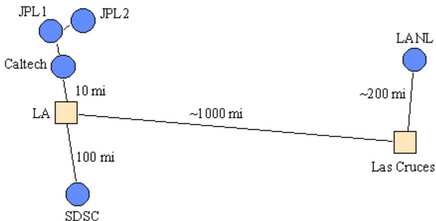
In Casa, the 2.5 Gbps links were divided into 16 SONET OC-3c 155 Mbps logical channels, with 8 of these channels made available at each site to provide a 1.2 Gbps aggregate full duplex rate for use by the researchers. The testbed logical topology is shown in Figure 3-6. While the Los Angeles junction for the LANL SONET link in Figure 3-5 was much closer to Caltech than to SDSC, carrier provisioning considerations resulted in the continuation of this link to SDSC using
