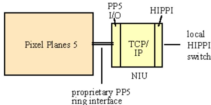
TCP/IP and UDP/IP protocol processing was supported using a 25 MHz SPARC processor, a custom multi-tasking kernel, and a custom protocol software implementation. Like the CBI, the NIU used hardware checksumming and flow-through data storage.
